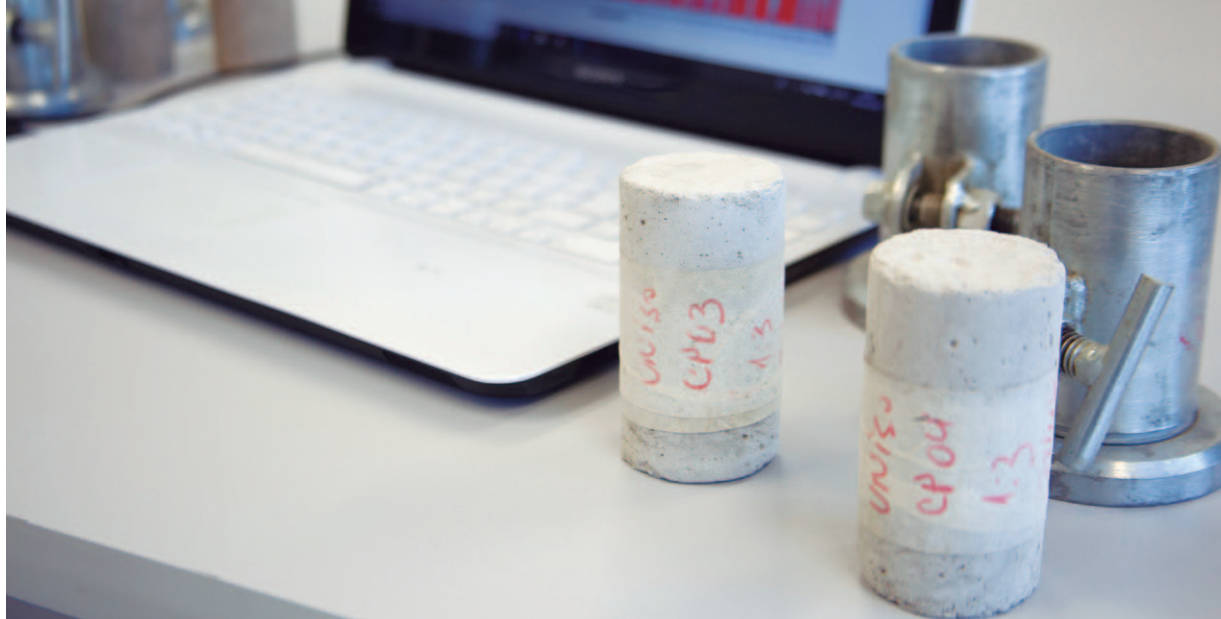
Corpos de prova produzidos no laboratório de Materiais de Construção Civil da Uniso Cylindrical specimens made of cement were produced for testing at Uniso's Laboratory of Construction Materials
